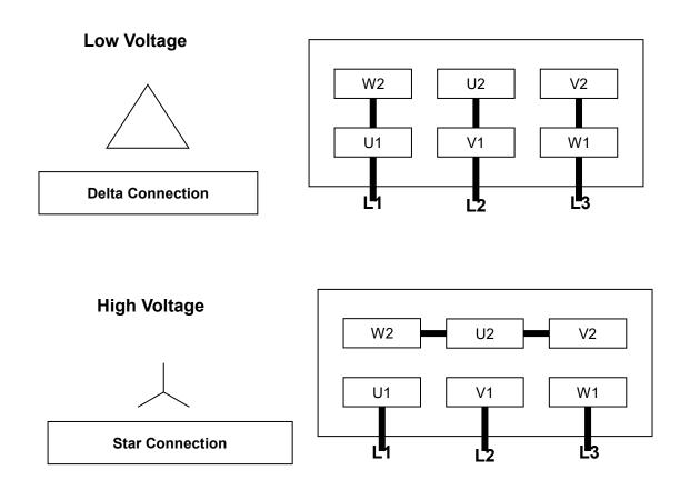
The motor must be connected according to the electrical codes through a fused switch in order to protect the motor against electrical or mechanical overload conditions. The overload of the motor starter must be set at a level equal to the full load motor current listed on the motor nameplate.
