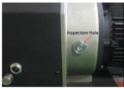
Inspection hole through G1" plug: Check the coupling and fan through this hole regularly. (The endoscope (WireCam) can be used with Smart Phone software)
